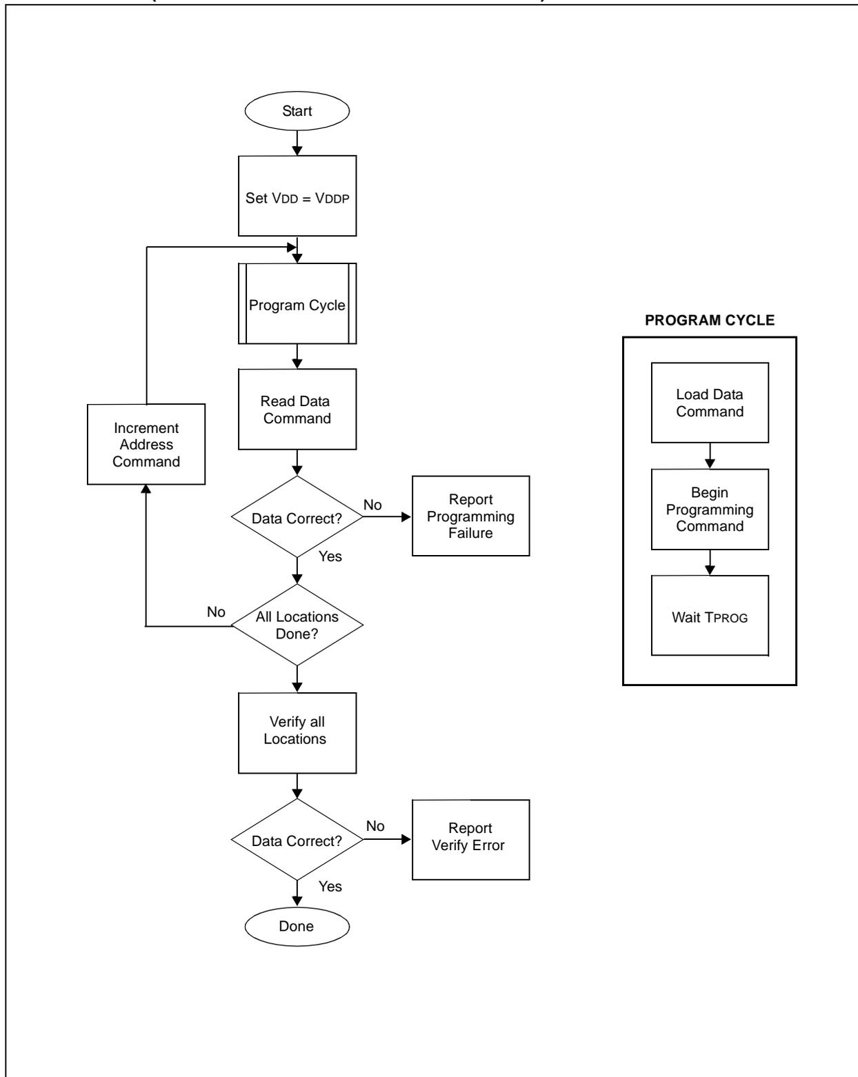
For PIC18 devices, an erase must be done separately before a write. Special commands that are triggered by writing to the configuration test area are used to clear blocks of program memory, the entire program memory, the configuration words, the data EEPROM or the entire device.
