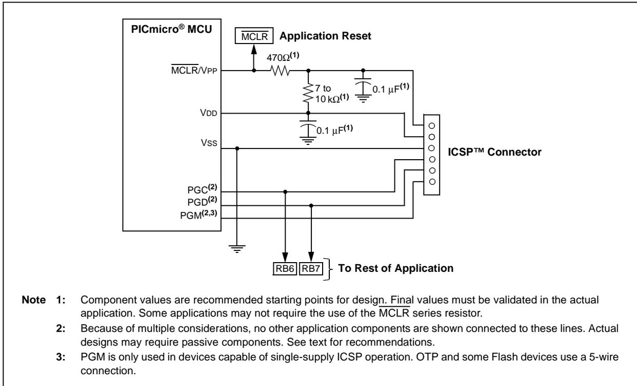
Some general circuit design guidelines are also provided in the *MPLAB ICD 2 User's Guide* (DS51331). While these are tailored to the requirements of the ICD interface, they also encompass the signalling requirements for the ICSP protocol. As a rule, any design that is signal compatible with ICD will also be compatible with the ICSP protocol, but not the other way around.
