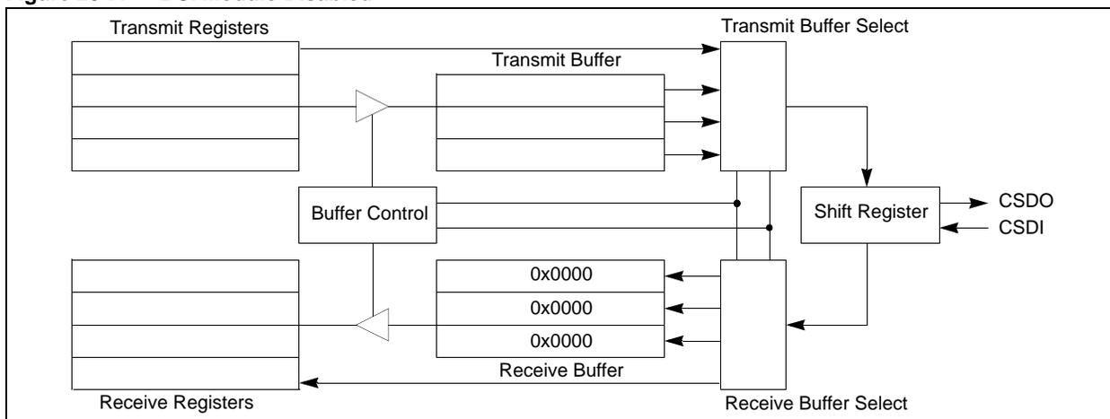
Figure 20-8 shows the state of the transmit registers after the application has written data to the TXBUF0 and TXBUF1 registers.
