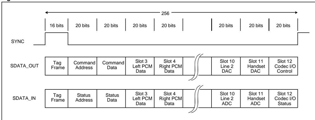
**Figure 20-35: Frame Sync Timing, AC-Link Start of Frame**
