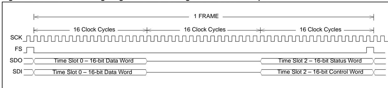
Since the codec transmits and receives the same number of time slots in a frame (TSCON = RSCON), the user application can write to successive TXBUF registers to transmit data and read from successive RXBUF registers.
