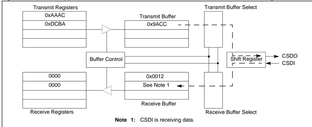
The module has completed transmit/receive operations of BLEN + 1 words, which causes an interrupt. The data in the receive buffers is copied to the RXBUFx registers. Figure 20-11 shows the data in the TXBUF0 is shifted to the shift register and the contents of the TXBUF1 register is copied to the transmit buffer. This cycle repeats with every DCI Interrupt.
