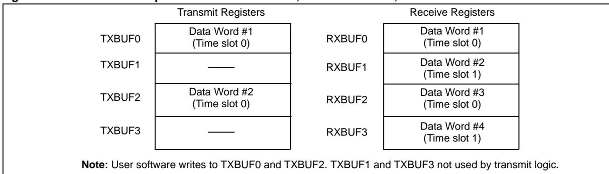
The buffer control resets to point to the first buffer location when BLEN + 1 buffers are written to and a CPU interrupt is generated, or TXBUF3 and RXBUF3 are processed and the buffer pointer must jump to the first buffer location.
