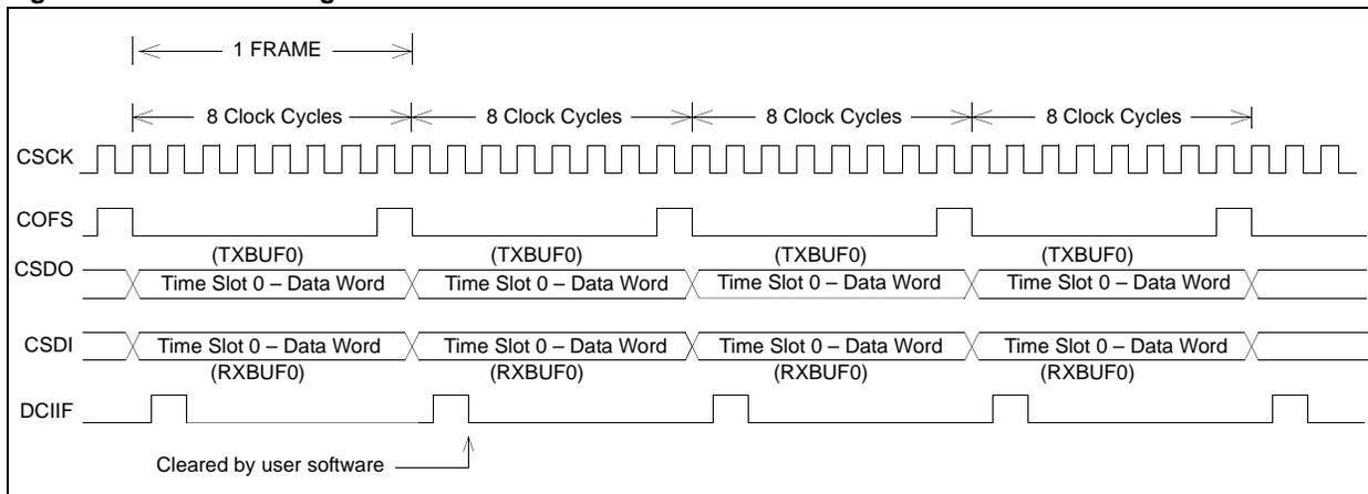
2. Assume  $BLEN<1:0> = 11$  (buffer four data words per interrupt) and  $TSCON = RSCON = 0x0001$ . This configuration causes the DCI to transmit or receive one data word at the beginning of every data frame. A CPU interrupt is generated after four data words are transmitted or received. This configuration is useful for block processing, where multiple data samples are processed at once. For details, refer to Figure 20-21.
