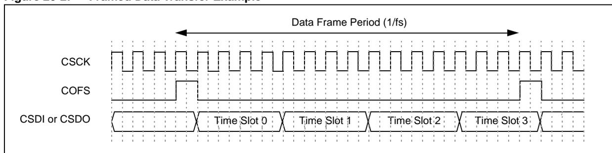
Figure 20-3 shows the timing for a typical data transfer with daisy-chained devices. This example uses a 16-fs SCK frequency and transfers two 8-bit data words per frame. After the FS pulse is detected, the first device in the chain transfers the first 8-bit data word and generates the FSO signal at the end of the transfer. The FSO signal begins the transfer of the second data word from the second device in the chain.
