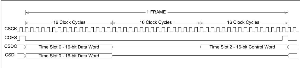
An alternate data alignment can be selected by setting the DJST control bit (DCICON2<5>). When DJST = 1, data transfers begin during the same serial clock cycle as the FS signal (refer to Figure 20-19).
