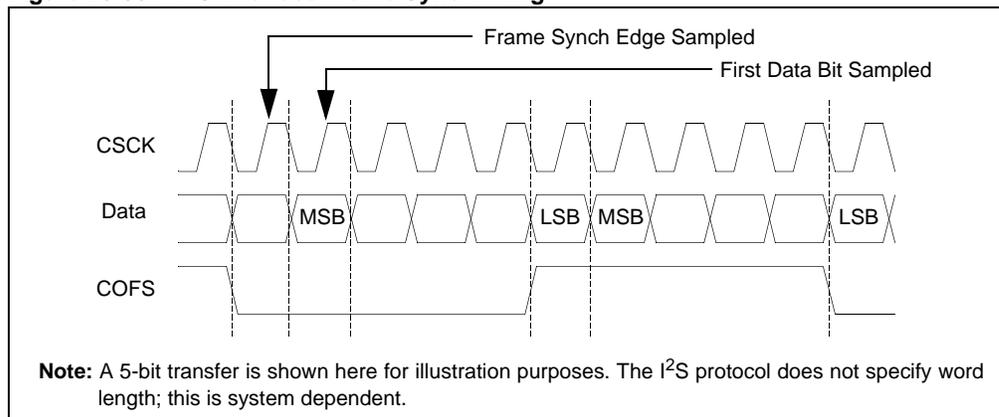
The DCI module is configured for I<sup>2</sup>S mode by writing a value of 01h to the COFSM<1:0> control bits in the DCICON1 SFR. When operating in the I<sup>2</sup>S mode, the DCI module generates frame synchronization signals with a 50% duty cycle. Each edge of the frame synchronization signal marks the boundary of a new data word transfer. The user software must also select the frame length and data word size using the COFSG and WS control bits in DCICON2.
