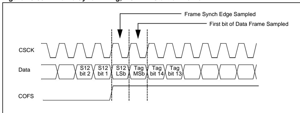
The DCI module has two operating modes for the AC-Link protocol to accommodate the 20-bit data time slots. These operating modes are selected using the COFSM control bits (DCICON1<1:0>).
