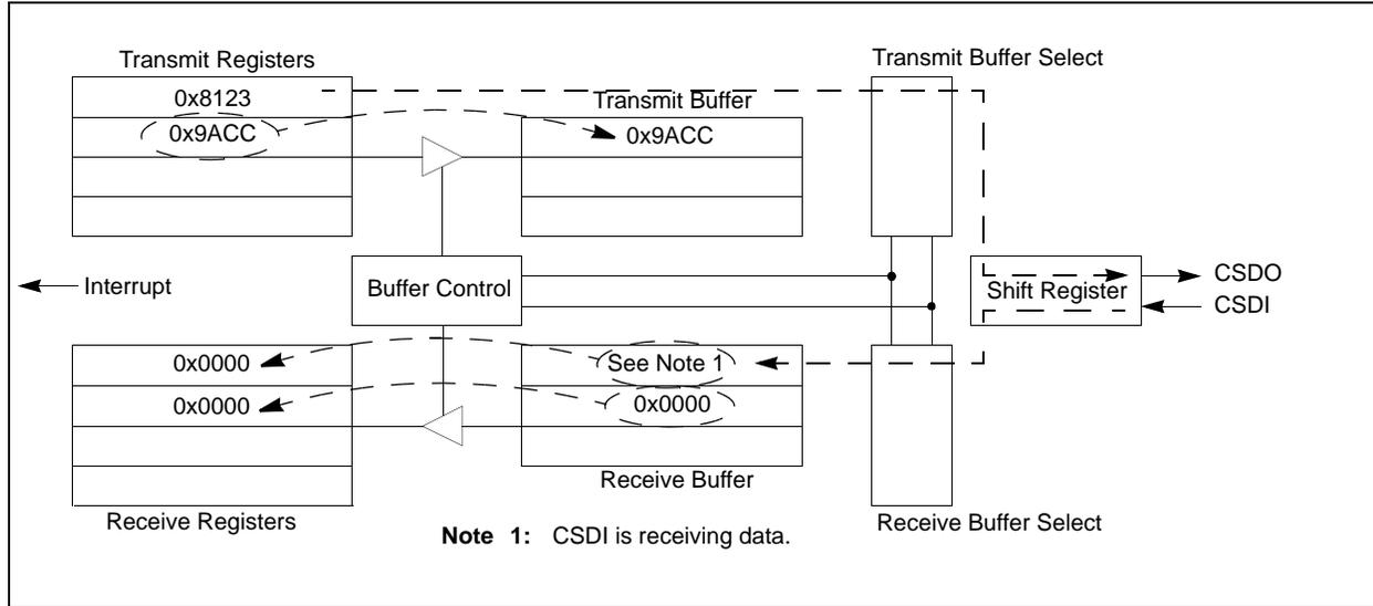
The user application writes new data to TXBUF0 and TXBUF1. Note that writing data to the TXBUFx register does not affect the current transmit operation. The second data word is shifted to the shift register. Figure 20-10 shows a new data word is received over the CSDI line into the Receive buffers.
