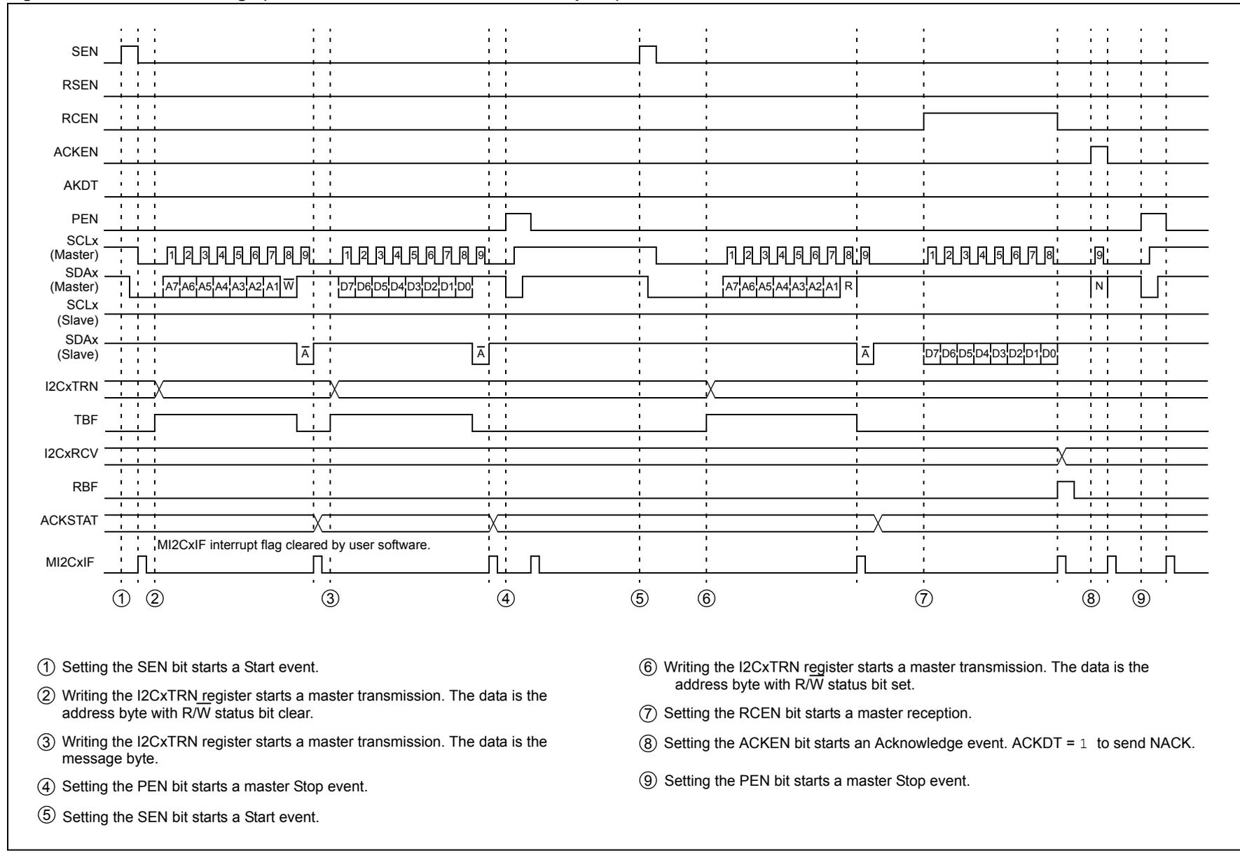
**Figure 19-16: Master Message (10-Bit Transmission)**
