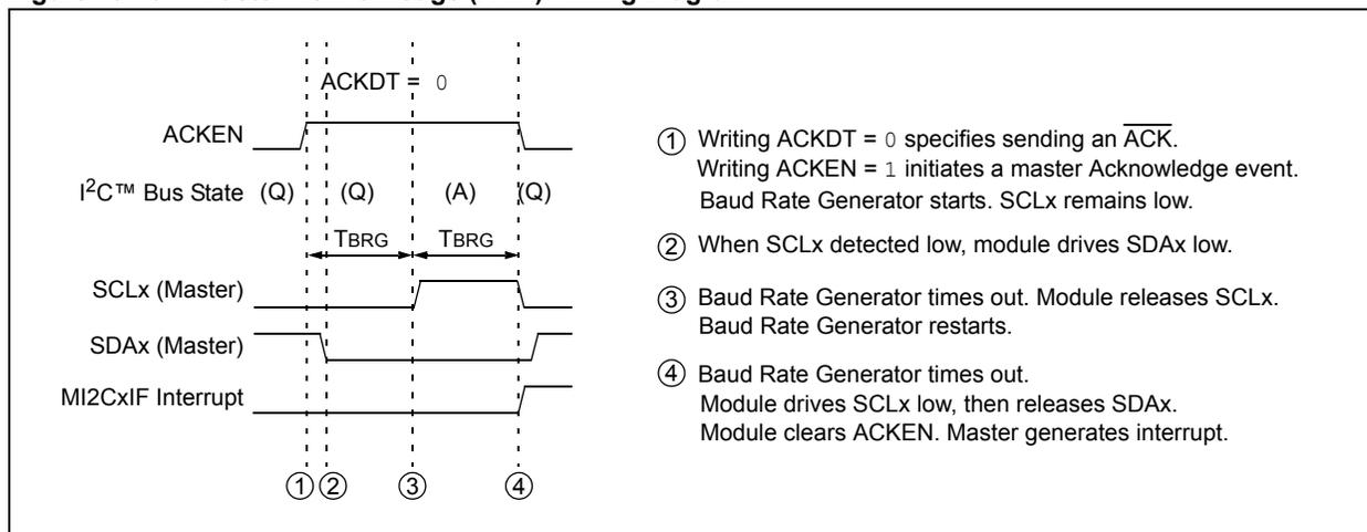
**Figure 19-11: Master Not Acknowledge (NACK) Timing Diagram**
