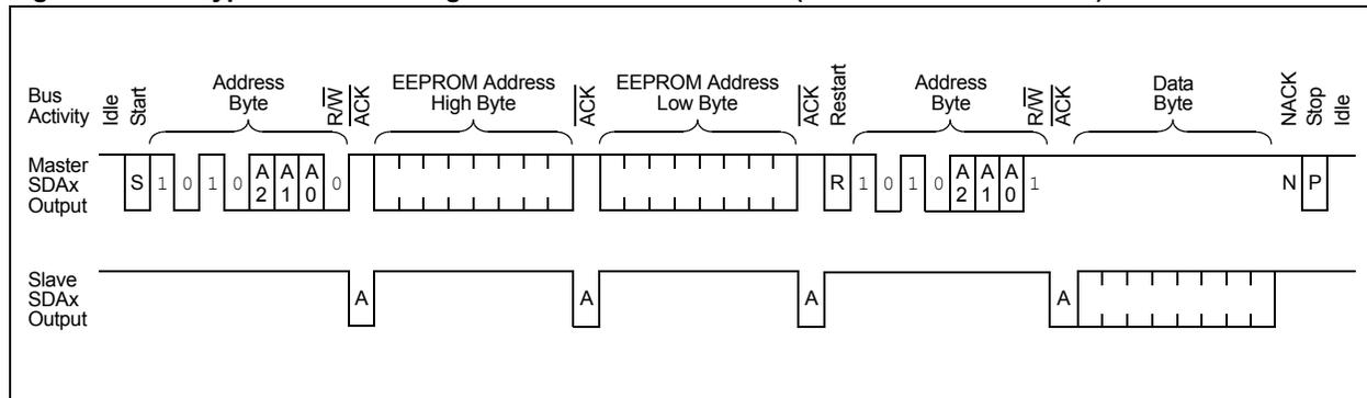
The I<sup>2</sup>C module supports Master mode communication with the inclusion of Start and Stop generators, data byte transmission, data byte reception, Acknowledge generator and a Baud Rate Generator. Generally, the software will write to a control register to start a particular step, then wait for an interrupt or poll status to wait for completion.
