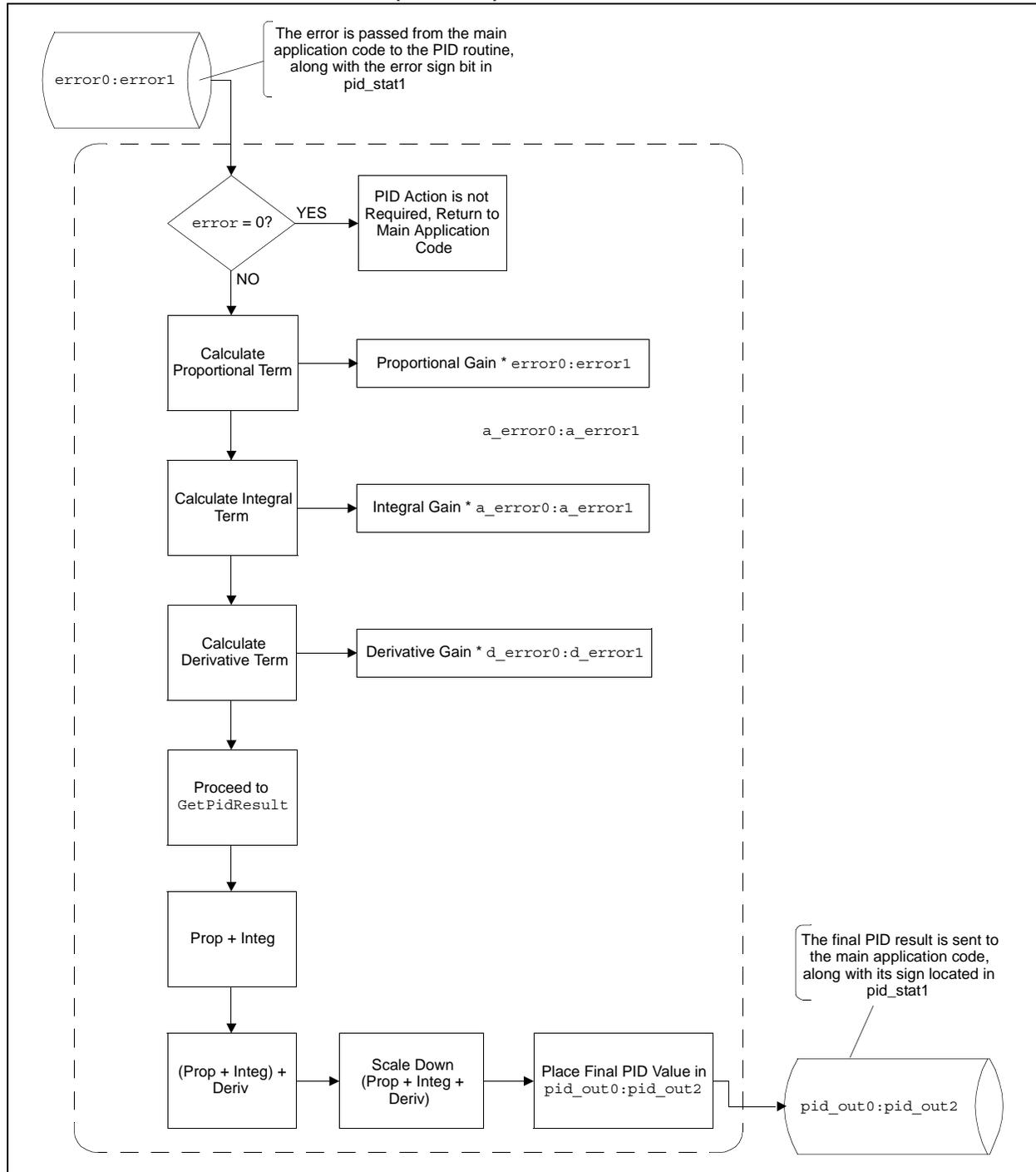
**FIGURE 4: PID INTERRUPT ROUTINE (PidInterrupt)**
