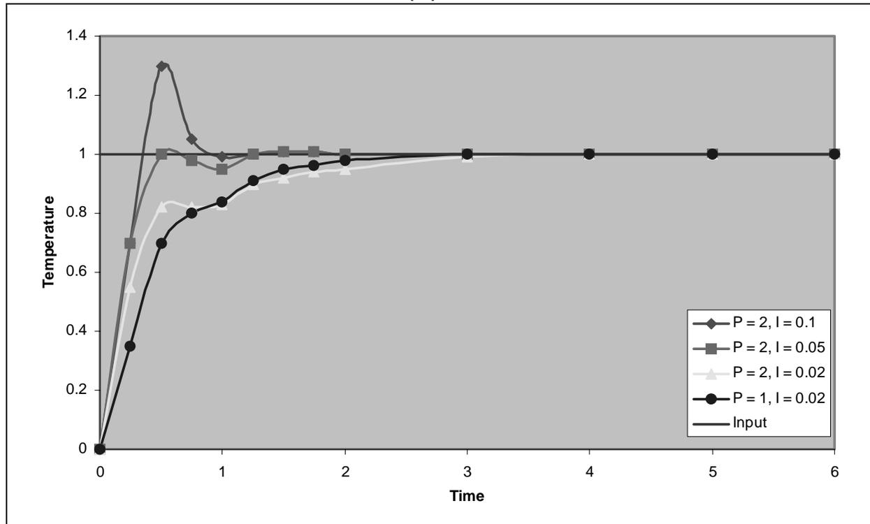
Figure 7 shows the graphic response of a PID Controller. This graph is very similar to the PI graph (Figure 6), except that the PID control takes half as long as the PI control to settle ( $t = 1.5$ ) as the Setpoint.
