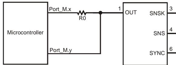
Electromechanical devices like relays will usually ignore the short HeartBeat pulse. The pulse also has too low a duty cycle to visibly affect LEDs. It can be filtered completely if desired, by adding an RC filter to the output, or if interfacing directly and only to a high-impedance CMOS input, by doing nothing or at most adding a small noncritical capacitor from OUT to Vss.
