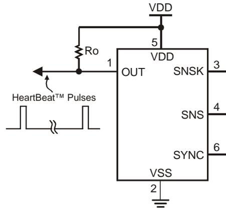
If the sensor is wired to a microcontroller as shown in [Figure 3-7](#), the microcontroller can reconfigure the load resistor to either Vss or Vdd depending on the output state of the QT100A, so that the pulses are evident in either state.
