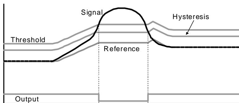
Once an object is sensed, the drift compensation mechanism ceases since the signal is legitimately high, and therefore should not cause the reference level to change.
