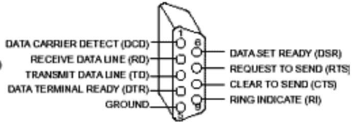
Figure 2. RS-232 Connector Pin Assignments
